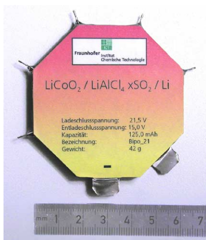
Fig. 4. Laboratory sample of a bipolar battery ( \text{Li}/\text{LiAlCl}_4 \times \text{SO}_2/\text{LiCoO}_2 ).
